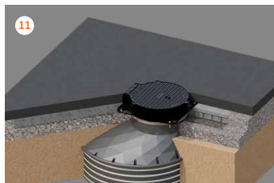
11 Install the final road pavement.
