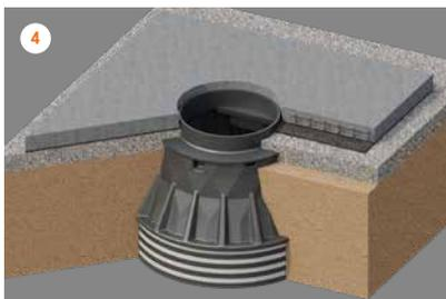
4 Add load balancing plate from reinforced concrete.
