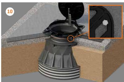
10 Fasten the cast iron cover at the corners with anchors bolts.
