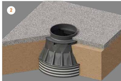
2 Add a layer of compacted crushed stone.
