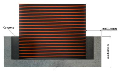
Concrete ring with closed bottom
