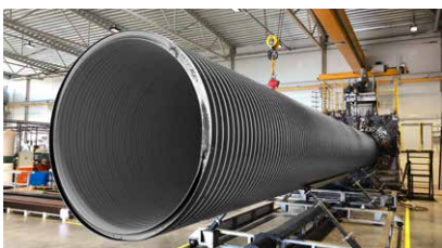
ID1600 mm PRODUCTION OF PIPES
