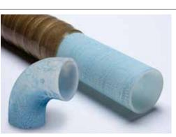
The PVDF HV-Liner from AGRU is an economical alternative to traditional fabric backed pipes. The surface-treated PVDF pipe has a three-dimensional surface structure which provides an optimal bonding to the FRP pipe. The piping systems are available in PVDF, PVDF-FLEX, and PVDF-el ESD. The pipes can be produced in diameters from 20 – 400 mm.
