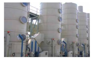
PP is the ideal material for the use in pickling plants, the chemical industry, and also for extremely aggressive waste water, as chemicals are used at high temperatures in these areas. The AGRU product range includes various PP polymer types:
