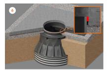
Install the sealing compound between the reinforced concrete plate and the service opening of the chamber.
