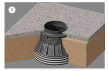
Add a layer of compacted crushed stone.
