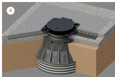
8 Install the cast iron cover.
