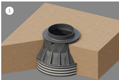
1 Trench compacted with backfill material.
