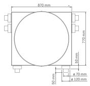
Application: Reserve and jointing well for communication cable pipes
