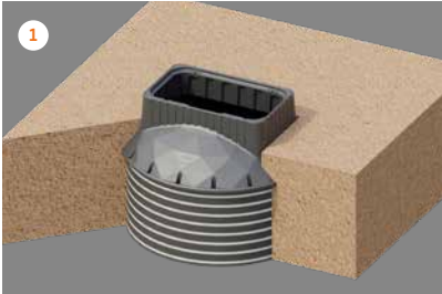
1 Trench compacted with backfill material.
