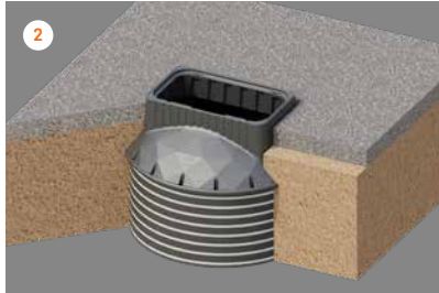
2 Add a layer of compacted crushed stone.
