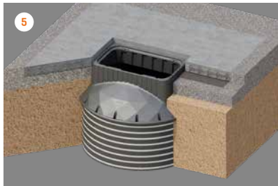
5 Add a layer of crushed stone around the reinforced concrete load balancing plate.
